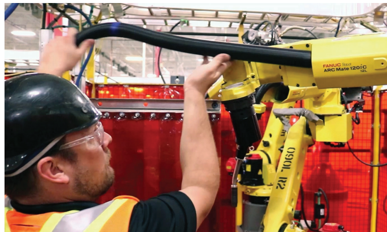
Pulsed welding waveforms can create wear on the through-arm robot's welding gun components, such as welding consumables and welding power cables.
