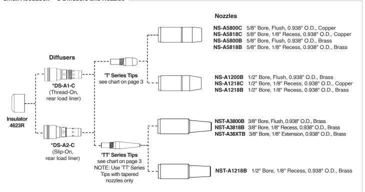
NOTE: \*Not engineered for error-proof liner replacement and flawless wire feeding. For use with Bernard® rear load liners. Refer to spec sheet SP-BER RLL for more information.
