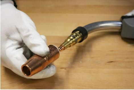
B. Loosen the gas diffuser.
