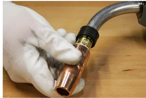
C. Place the power pin cap over the liner and thread onto power pin.
