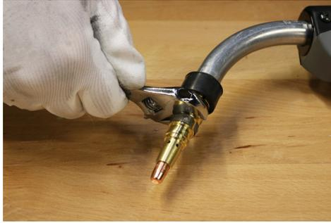
C. Remove the gas diffuser.
