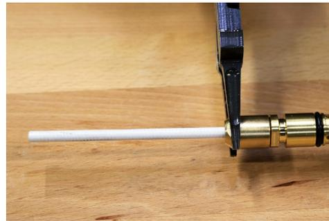
E. Holding the hex wrench as shown, tighten the set screw "finger tight" against the liner.
