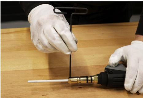
F. Next, hold the hex wrench by the handle and tighten the set screw an additional one-half turn to fully secure the liner.
