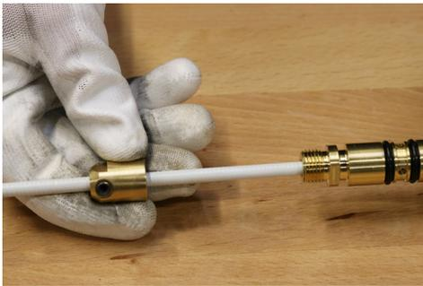
D. Tighten the cap snug against the power pin shoulder with welding pliers or appropriate wrench.
