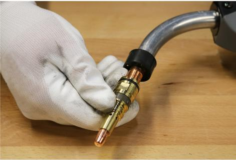
D. Loosen the set screw in the power pin cap and remove the cap from the rear of the gun.
