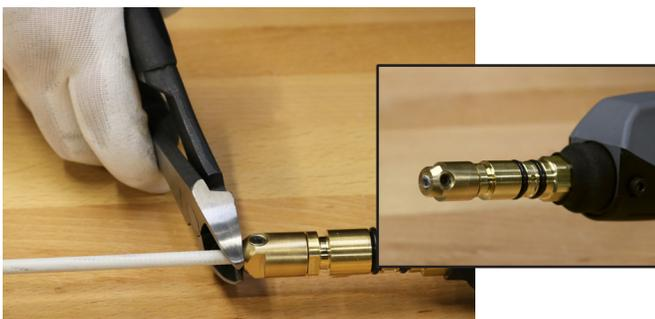
B. Insert a piece of welding wire into the liner to check for burrs or obstructions. If needed, loosen screw slightly until wire slides freely.
