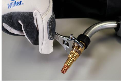
C. Remove the gas diffuser.
