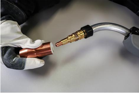
B. Loosen the gas diffuser.
