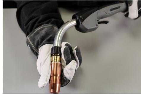
C. Identify the power pin to determine the appropriate power pin cap torque specification.
