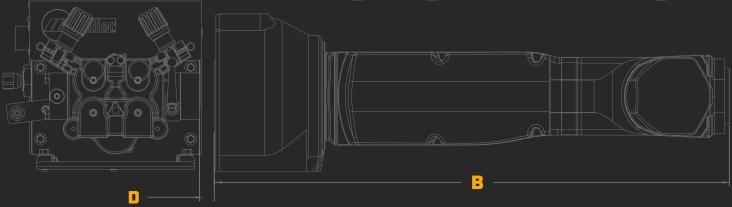
MEASURE THE LENGTH OF THE ROBOT ARM: INSERT A TAPE MEASURE THROUGH THE WRIST OF THE ROBOT AND MEASURE FROM THE END OF THE ROBOT ARM CASTING TO THE FACE PLATE ON THE WRIST  $\rightarrow$  DIMENSION "B".
