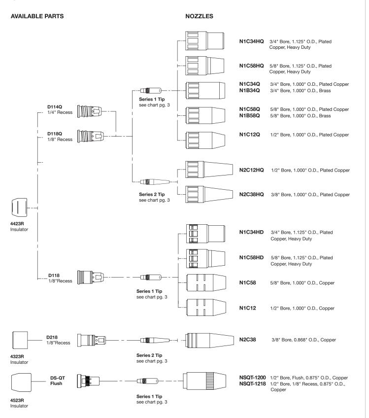
DIFFUSERS AND NOZZLES ARE AVAILABLE IN PACKAGES OF 10, INSULATORS IN PACKAGES OF 5 AND CONTACT TIPS IN PACKAGES OF 25  $^{\circ}$
